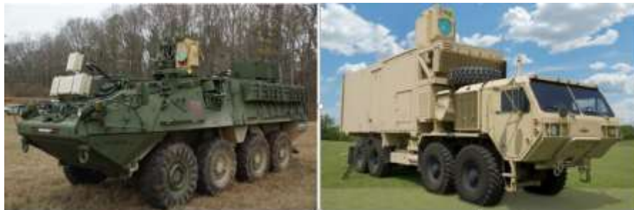
An early experimental laser-armed Stryker vehicle, the MEHEL (left) and an early Army HEL (High Energy Laser) Mobile Demonstrator (right)
